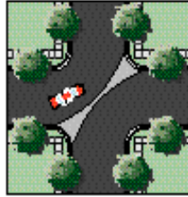
Diagonal Road Closure with Strip
