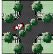
Diagonal Road Closure with Bollards
