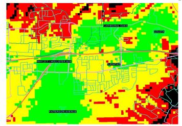
**Coverage** is best shown via coverage maps. RF engineers use tools that take into account terrain, vegetation, building types, and WCF specifics to model the existing coverage and prediction what we expect to see with the addition of a proposed WCF.
