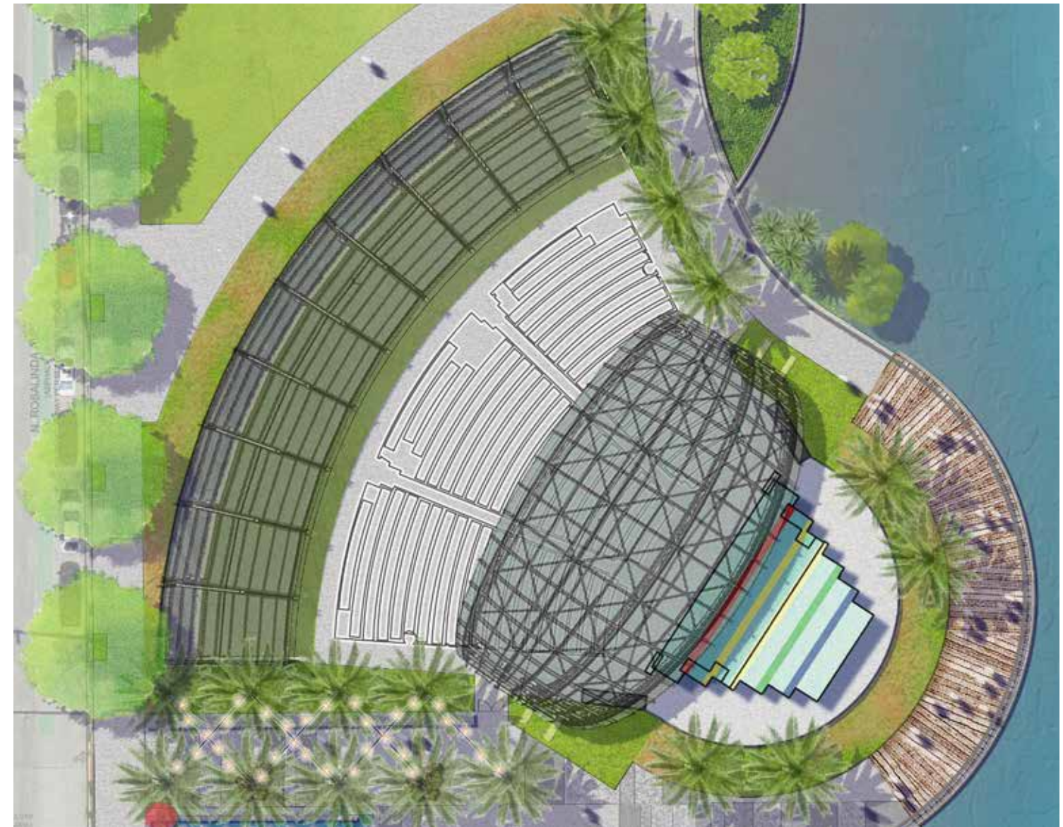
The improved Amphitheater space maintains the existing Band Shell and seating and enhances it with additional shade canopies in front of the Band Shell and a metal canopy covering an additional sloped lawn seating area.
